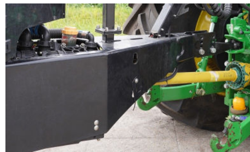
High hitch with 40 mm drawbar eye
